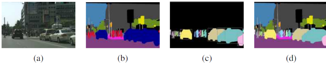
Figure 1: (a) Image, (b) Semantic segmentation, (c) Instance segmentation, (d) Panoptic segmentation
